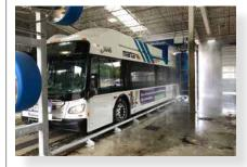
Transit-Master. For buses with front mounted bicycle racks. Dryer system.
